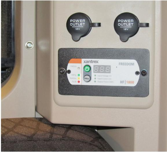
Power inverters – the devices that convert standard battery (DC) power to AC household power – are becoming more commonplace in the trucking industry.
