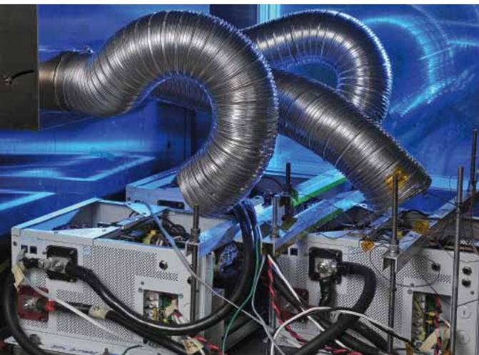
▲ Xantrex Freedom SW inverter-charger at test
