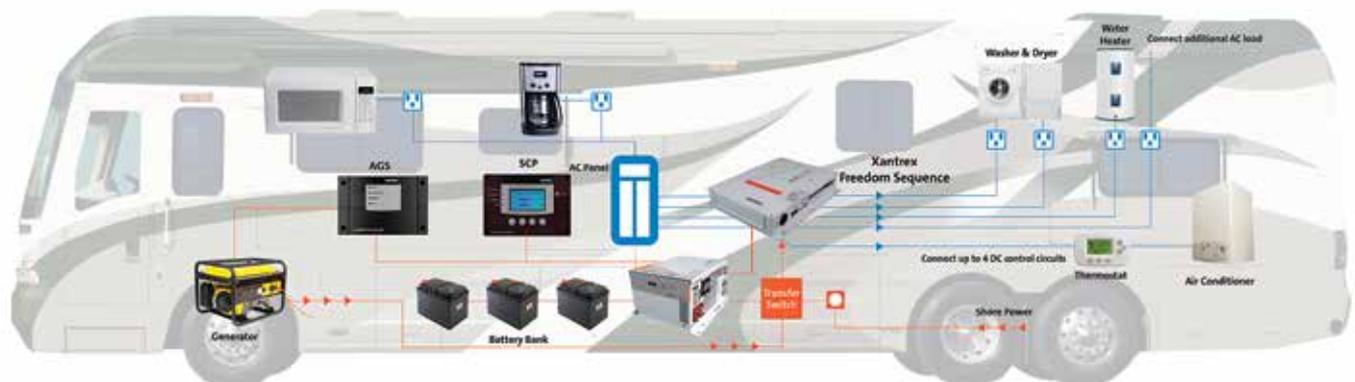
Xantrex Freedom Sequence Intelligent Power Manager offers an integrated power system where all onboard components can communicate with each other and be managed through a single control panel.
