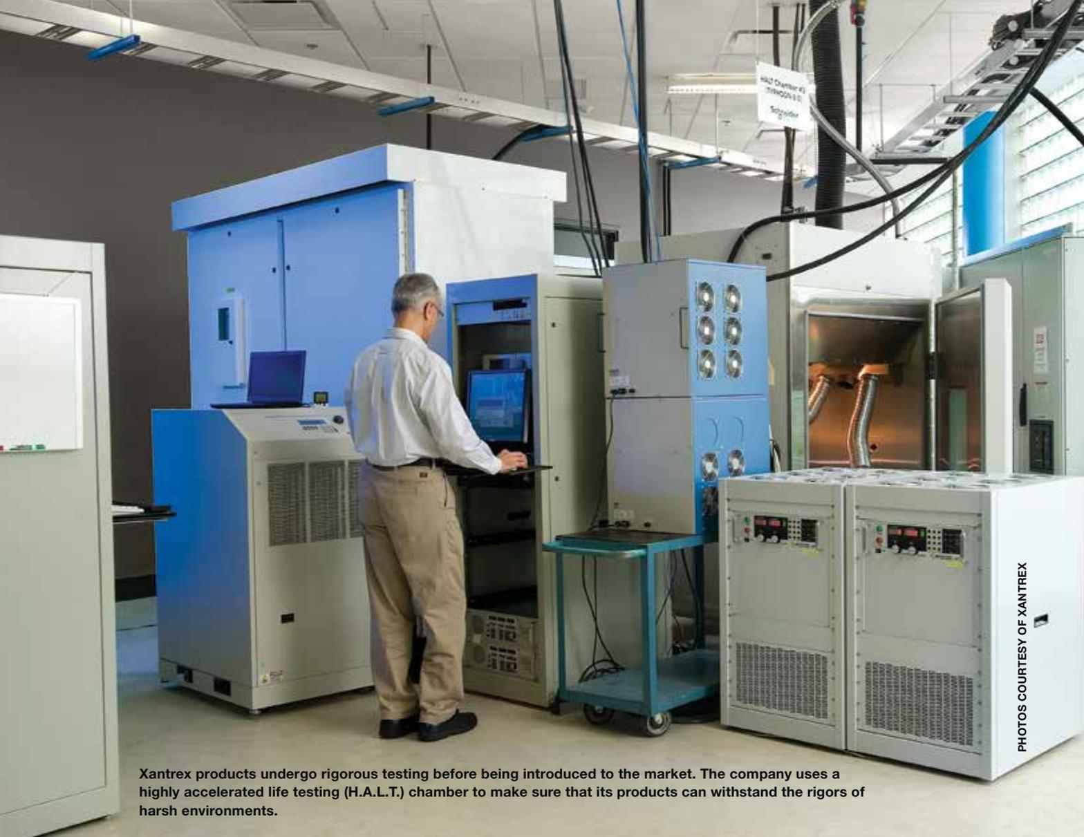
Xantrex products undergo rigorous testing before being introduced to the market. The company uses a highly accelerated life testing (H.A.L.T.) chamber to make sure that its products can withstand the rigors of harsh environments.
