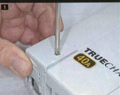
[1] Removing the plate in the corner of the unit provides access to the power leads. [2] The wires were connected to a 12-gauge extension cord, which took a little maneuvering [3] to get all terminals and wires contained in the tight space.
