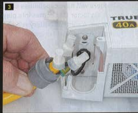
[1] Removing the plate in the corner of the unit provides access to the power leads. [2] The wires were connected to a 12-gauge extension cord, which took a little maneuvering [3] to get all terminals and wires contained in the tight space.
