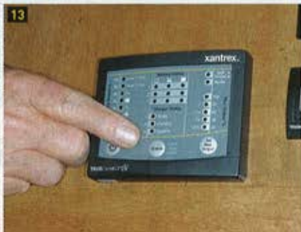
[13] The remote panel is installed in a convenient location inside the RV. Controls and indicator lights mimic the panel [14] on the outside of the charger housing. [15] The temperature sensor is connected to the negative post of the battery.
