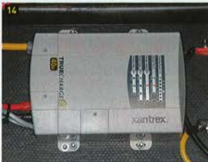
[13] The remote panel is installed in a convenient location inside the RV. Controls and indicator lights mimic the panel [14] on the outside of the charger housing. [15] The temperature sensor is connected to the negative post of the battery.
