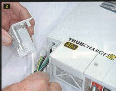
[1] Removing the plate in the corner of the unit provides access to the power leads. [2] The wires were connected to a 12-gauge extension cord, which took a little maneuvering [3] to get all terminals and wires contained in the tight space.
