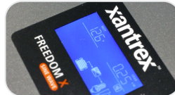
View AC & battery current, % status bar for inverter output on the onboard display
